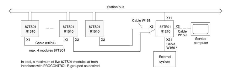
\* For connecting the external system, a W160 cable with a 25-pole HDP20 pin-type connector can be used.
