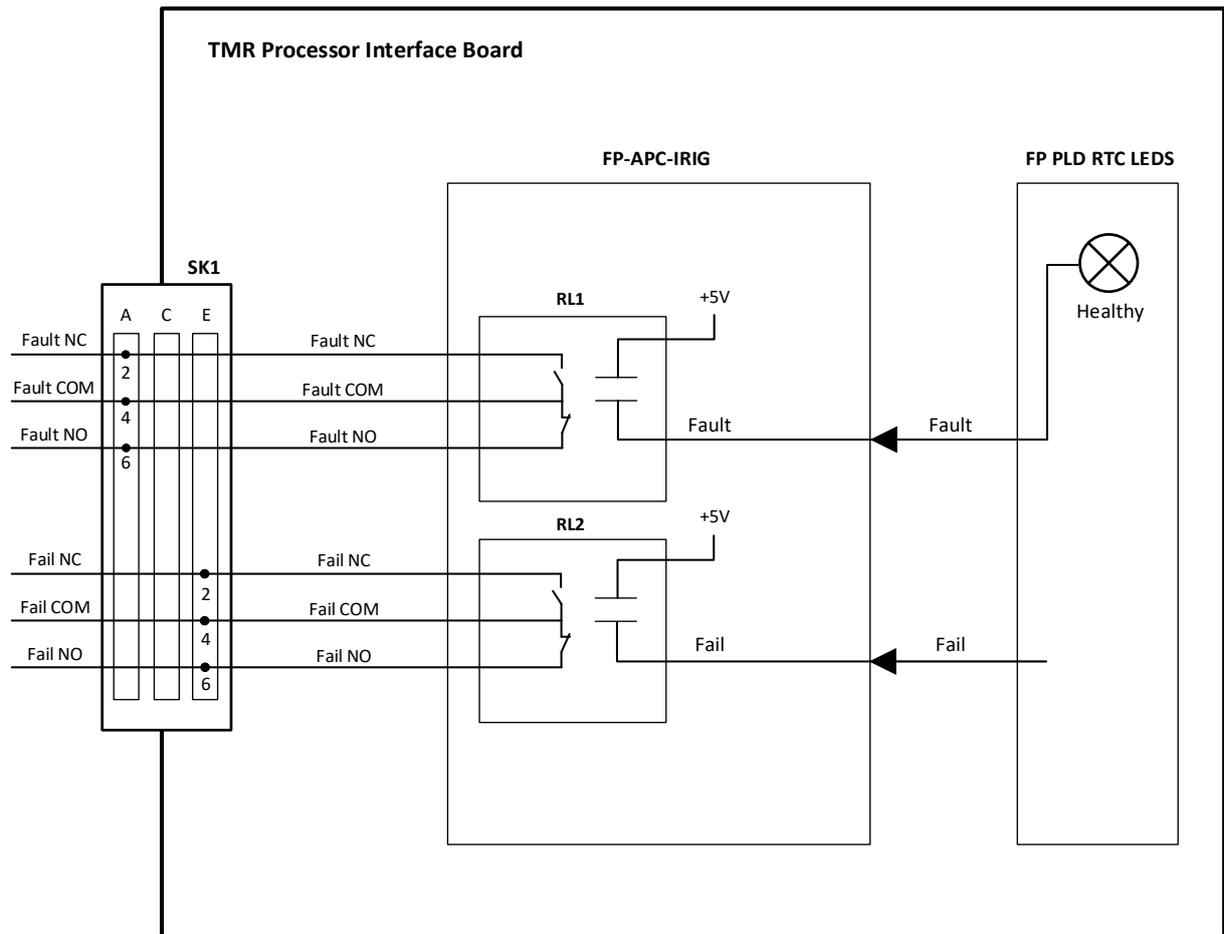
**Figure 2 Fault/Fail Relays**
