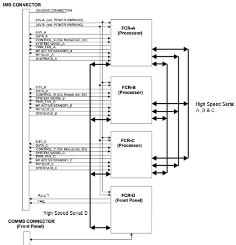
Figure 3 Functional Block Diagram showing Trusted TMR Processor Communications
